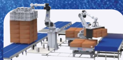
Palletizing station with robotic arm
