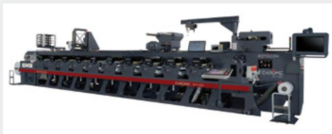
*for high efficiency and flexibility, will also be demonstrated. Its modular design allows for customised configurations as converters' needs grow, including hot and cold foil, embossing, multilayer labels, in-mould labelling, and screen printing.*
