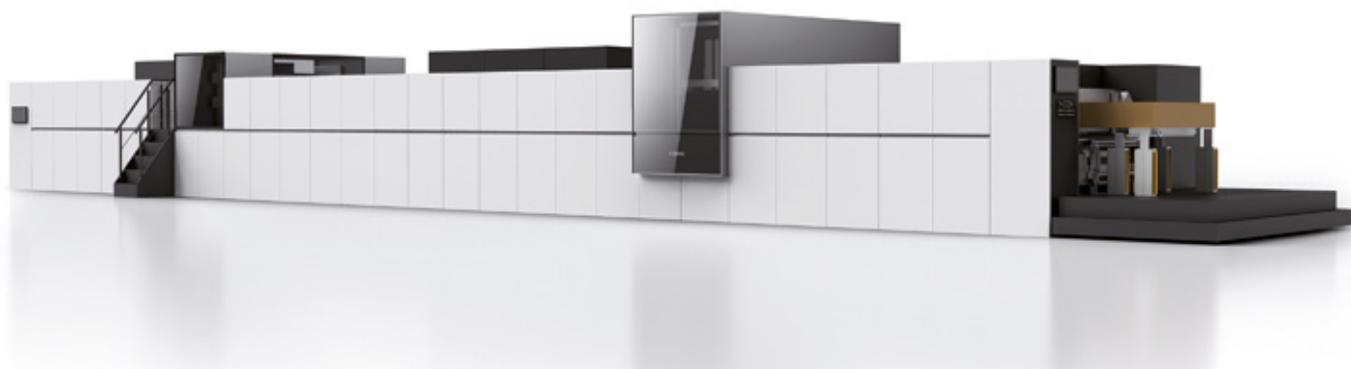
*adhesion to the substrate and reduces dot gain: the primer is applied by a printhead to the surface of the paper before the actual printing process and only where it will be printed afterwards. It prepares the surface of the paper without altering its texture so that pigment particles can be quickly fixed to it. Without any upfront drying section the 4-7 colors will be printed in a wet-in-wet process reducing the heat load of the board.*
