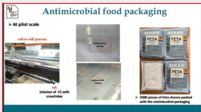
some tests have also demonstrated the validity of flexo printing. The use of multifunctional thin layers would allow the replacement of multilayer and heavy structures, thus reducing the amount of upstream packaging materials, while maintaining (or even improving) the functional properties of the final package, pursuing the goal of extending the overall shelf life and optimizing the packaging.
