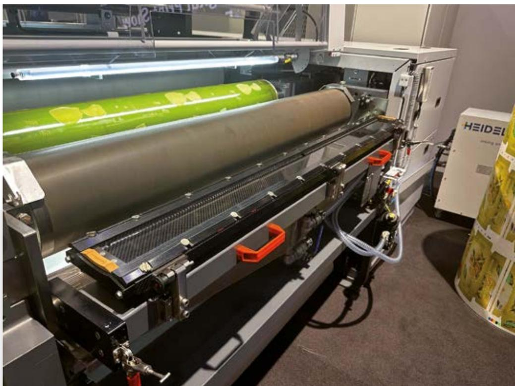
are equipped with an automatic pressure management system, controlled via software by the machine itself. This system is designed to automatically compensate for blade wear, ensuring constant and optimal performance over time.
