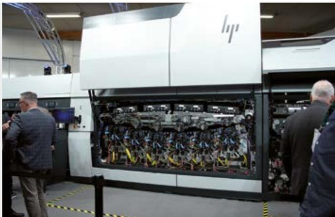
meters/min with a resolution of 1600 dpi; as regards substrates thickness can vary from 12 to 450 micron, exploiting the in line primer application unit. For even greater productivity, ABG's nonstop winding solution - specifically developed to run with the HP Indigo V12 digital press was also demonstrated at Labelexpo.
