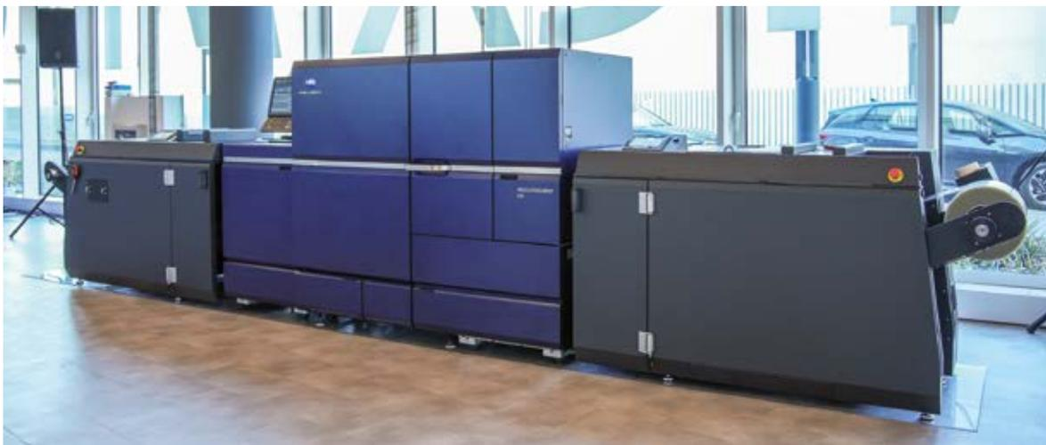
is now 2400x3600 dpi, doubling that of AccurioLabel 230, so printing quality is comparable to offset, also thanks to the choice of 14 different types of screens. An absolute novelty for the world of Konica
