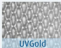
*UV Gold* engraving has a very low ratio between volume and cell depth, making it suitable for highly viscous (UV) inks. It is extremely easy to clean. Maximum achievable volume for a given screen count is increased by 20% to 30%.
