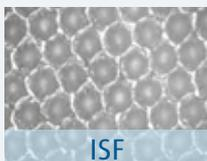
ISF engraving (Ink Spitting-Free) is effective in preventing spitting. The use of channel engraving allows the ink to flow within the engraved channel across the anilox surface, decreasing the ink build-up and hydraulic pressure of the blade.
