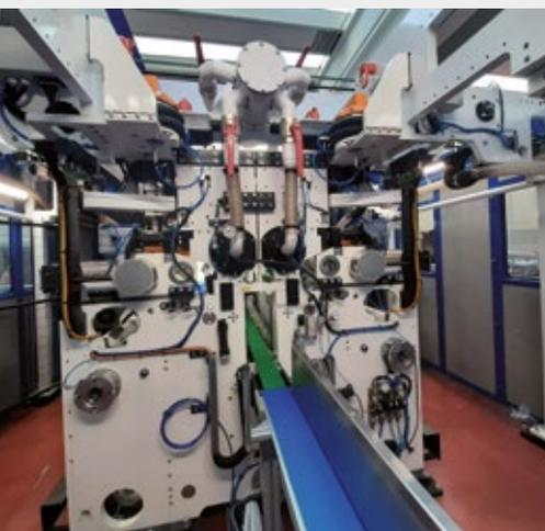
*Patented by Körber Business Area Tissue, the MTC ITF Change has only two folding rolls, which the cutting function is incorporated into.*
