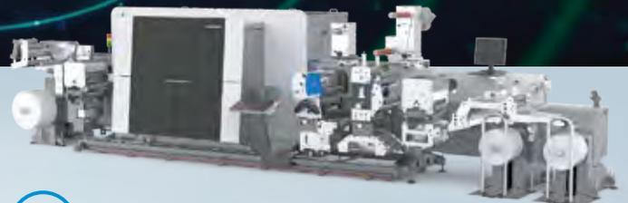
**D3** 4-colour inkjet printing system with integrated inline finishing modules\*
