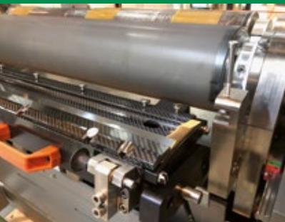
of error. BFT CARBON, on the other hand, will be presenting the latest in carbon fibre doctoring chambers dedicated not only to the flexographic world, but also to offset and rotogravure. On this occasion, the latest doctor blade chamber models dedicated to the corrugated sector will be presented, ready to be quickly installed on the machines of the most popular manufacturers.
