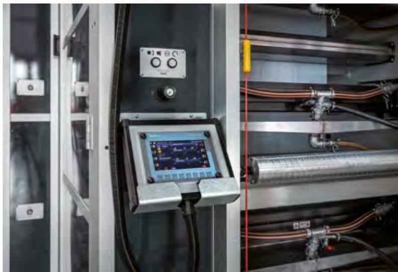
doors equipped with all accident prevention safety systems. An important feature is the positioning of the electrical part on the upper deck of the machine, to reduce the footprint of the machine itself.
