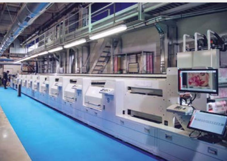
value to the work (double pass with black, unit dedicated to screen printing and one to cold foil and finally a classic four-color process to complete the 8 steps possible
