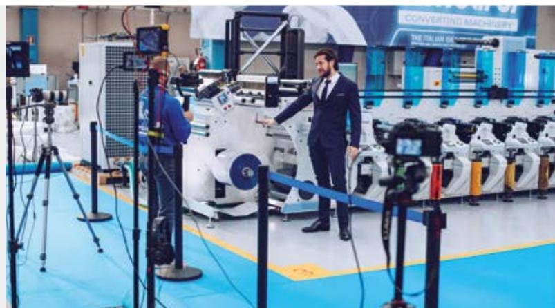
tion Lombardi's best-selling technology, the Synchroline 430 for flexible packaging printing, 250 lines installed in 45 countries around the world. Fully servo-motorized machine capable of printing on different materials, such as paper, film, shrinkable material, aluminum, adhesive paper, cardboard with material thicknesses from 50 up to 500 microns, dedicated to packaging but also allows the printing of labels and is therefore an extremely versatile technology.
