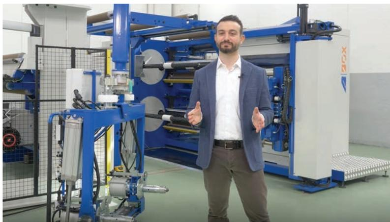
a very versatile accessory, namely the rotating reel unloader, which allows manual unloading for lighter reels, servo-assisted unloading, controlled by the operator, for the transfer of the reels from the arms of the reel unloader to the manipulator and to the final palletizing phase, and finally
