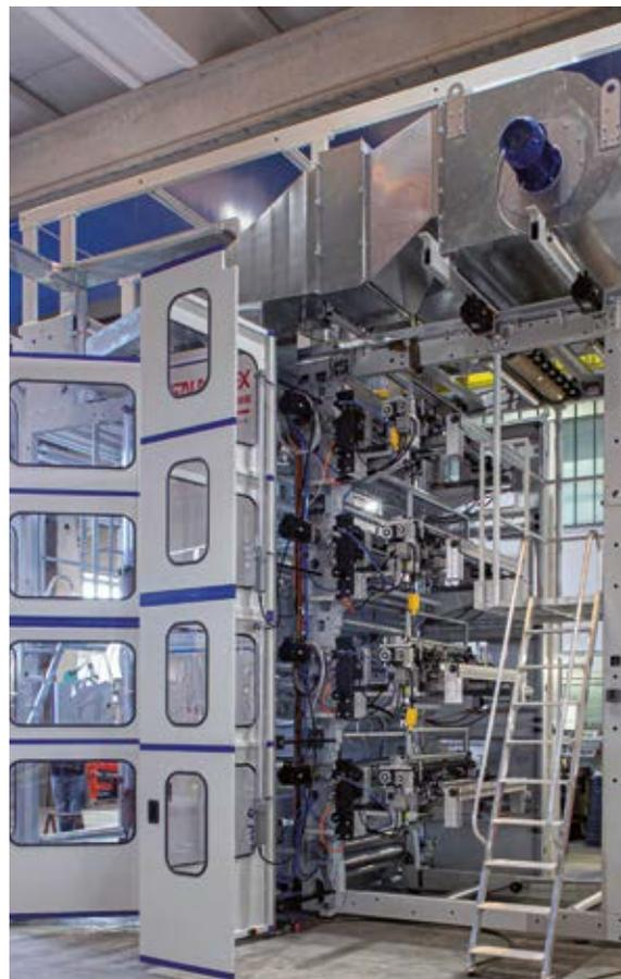
*Saldoflex has understood that finding the right partners can bring great results: from the technological synergy with Bosch Rexroth was born LEAF-S8, a central drum flexo machine based on artificial intelligence and Machine Learning, able to regulate set-up pressure automatically and quickly,*
