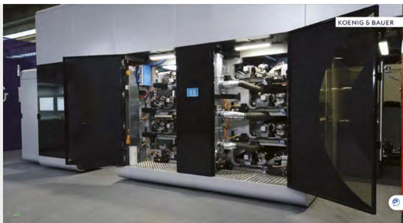
virtual registration marks with the printed ones with a simple finger touch to calibrate the register and lock it in the most precise position. The operation is simple and in a very short time is performed for all colors to print. As the machine speed is increased, the register marks will remain perfectly stable. At this point the Evo XC is ready to print
