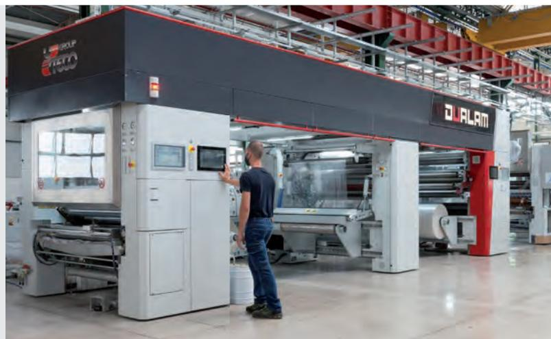
1 winder. The whole process starts from the solventless unit where there are 2 steel rollers to dose the gap and the adhesive, 1 sleeve that is easy to manage and very quick for job changes for transfer to next steel roller where converges the primary film which is coated with adhesive", says Bicego in front of the new Dualam managed by his colleague Simone Rossignoli, senior
