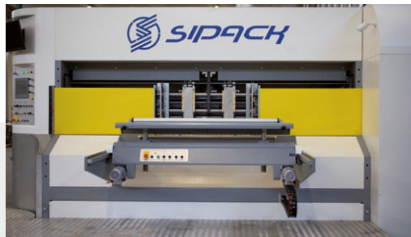
positioned, even if big, even when held by just one operator. Quality printing requires systems that reduce ink consumption. For this reason, Sipack has chosen to install carbon chambers doctor blades. With a market growing on ambition and quality, with frequent changeovers, printing systems that help to economize are even more relevant and Sipack responds to these challenges with smarter and user friendly machineries, bringing real value to the producer.
