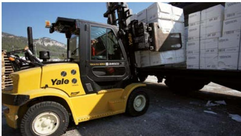
represent a challenge to the handling machines. If they permeate into the inner workings of a truck, they can cause overheating due to clogged cooling filters and therefore the temporary loss of an indispensable asset. Moreover, the risk of fire is amplified, as paper is highly combustible.
