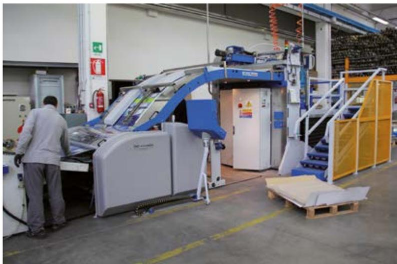
*both the front and side position of the sheet just before having to register it with the substrate base sheet. The base sheet is also handled in its longitudinal and transverse position. The register is thus performed in an extremely precise and "on the fly" way without any need to stop and re-accelerate the sheets themselves. The passage of the sheet becomes constant and the speed of the machine increases significantly.*
