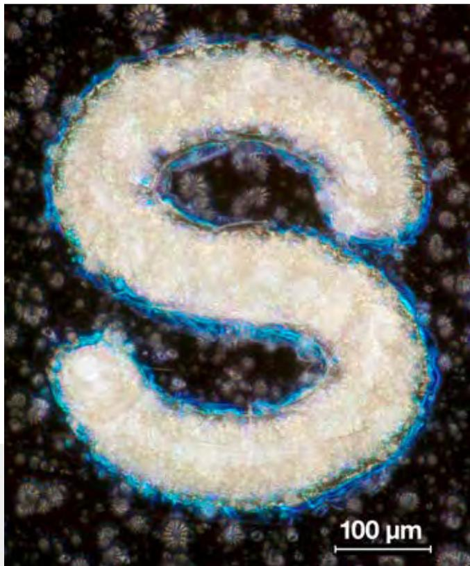
have a layer thickness of 50 microns. This minimized coating thickness makes it possible to maximize font resolution, resulting in enhanced microscopic delicacy.
