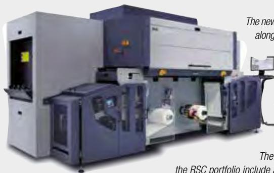
The new Tau RSCi, on display along with the Tau 330 RSC and RSC-E presses, offers print widths of 330, 420 or 508 mm and a print speed of up to 100 linear meters per minute.
