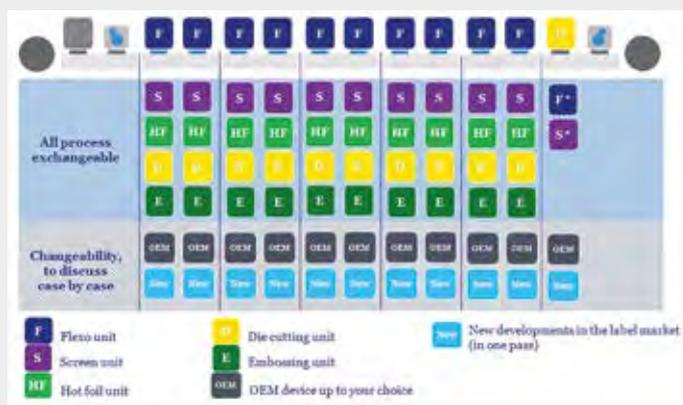
stainability, but also for potential savings. In this case for the Gallus Labelmaster, the web travel from printing unit to printing unit is 1.4 m. This is made possible by the arrangement of all essential processes on the primary level, whereby no change to another level is necessary. The use of a screen printing unit on a rail, for example, causes an additional path of 4 to 6 meters. The arrangement of the
