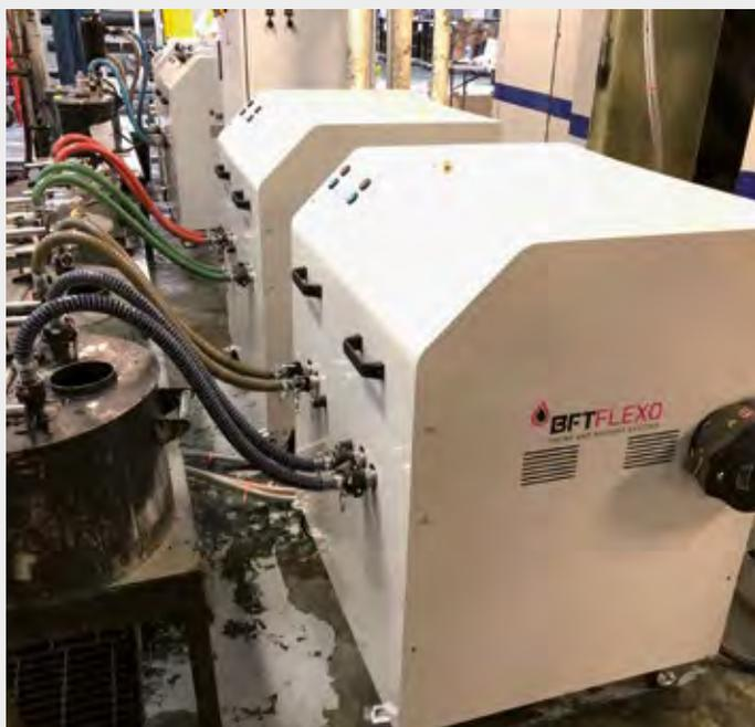
*"The inking and washing system we have designed is very flexible and can also be managed as an integrated part of the printing machine itself that can control it directly", says Alberto Ferrara, BFT Flexo technical director.*
