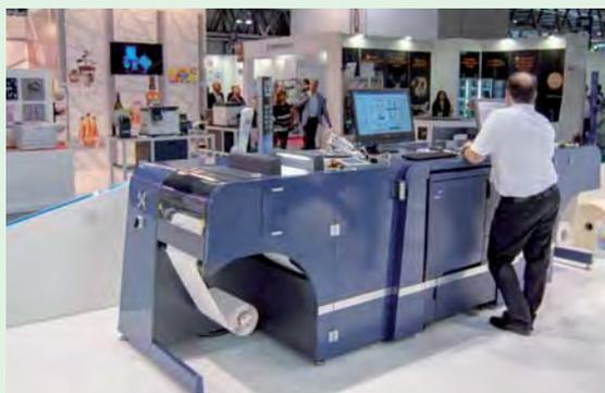
*solution allows you to make finishings in the preferred order, varnishing - foil or vice versa and even the finer details of the images will be perfect thanks to AIS, the automatic register system for varnish and hot foil, which does not require marks and therefore reduces the time spent for the registration process by 80%.*
