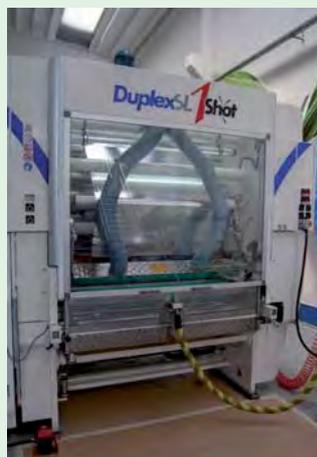
*presented by the partnership between Nordmeccanica and Dow in these two years has revolutionized the lamination concept, drastically reducing production times: 90 minutes from laminating to cutting, thanks to the special composition of Symbiex™ adhesive, developed by Dow and the technology implemented on the laminating machine Duplex SL One Shot™ by Nordmeccanica.*
