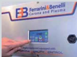
treatment data from the generator to the PC and produce process quality certificates. Ferrarini & Benelli has developed two systems for treating 3D objects or small flat surfaces that can be integrated in-line, or used in the laboratory for testing. In Air Plasma and In Air Corona are composed of a high frequency digital generator with integrated transformer and one or more dispensing heads.
