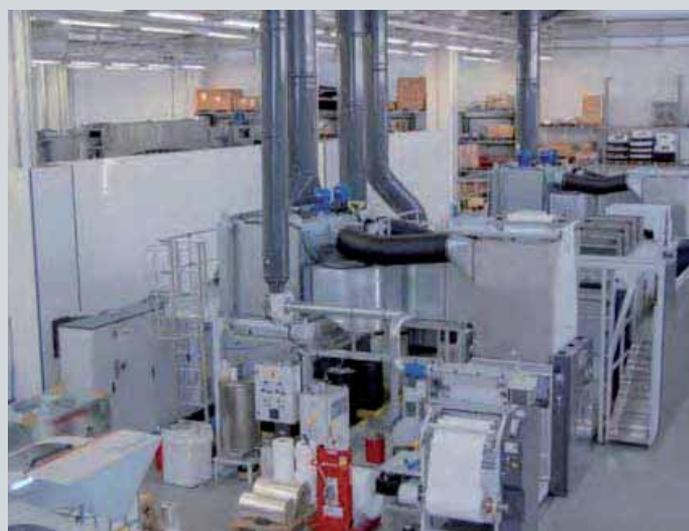
*gle-shaft unwinder; gravure unit with anilox and closed chamber doctor blade to apply the primer to the flexible substrate which is dried with hot air; then the 4-ink*
