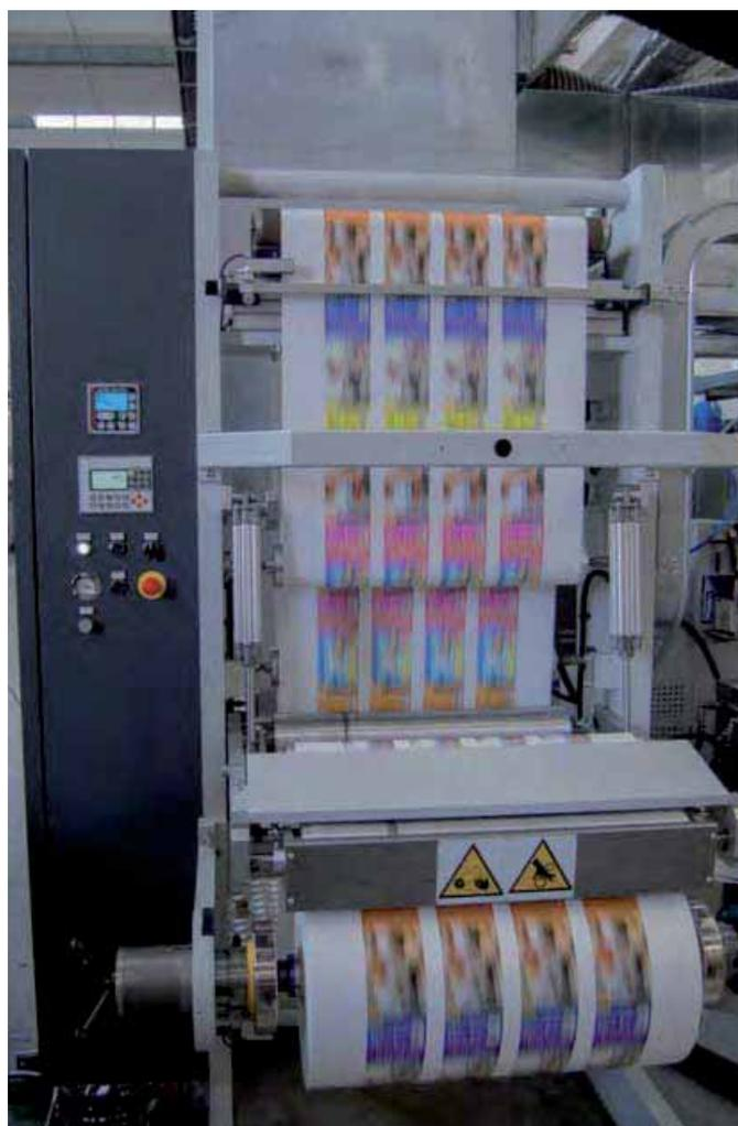
*a flexible film for packaging printed on a flexo printing machine, the Uteco Onyx 812, optimized for advanced WetFlex printing using EB inks with Uteco EB2 technology, equipped with two inkjet heads Kodak Prosper, the S20 model, which prints in black plus one color. Subsequently, at Drupa 2016, Uteco/Kodak Sapphire was exhibited,*
